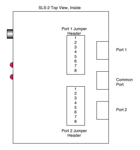
Any rewiring you perform will require you to de-solder the wires on the jumper headers and re-solder in a different configuration.
